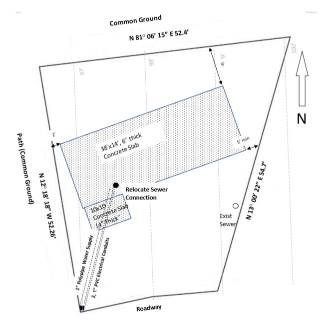
Notes: Concrete to be 4,000 psi minimum Install Welded Wire Mesh or No 4 Rebar spaced 12" both directions.
